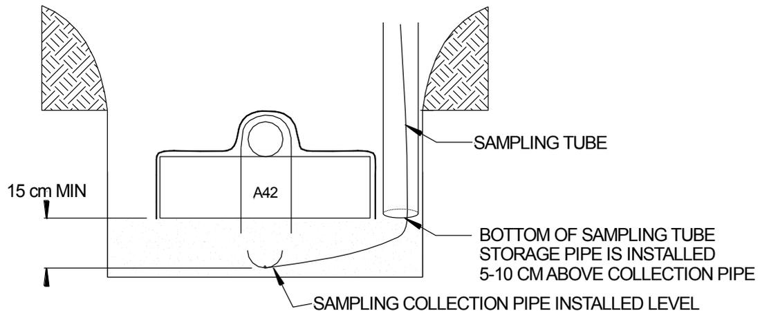
*Note: Separation distance from the bottom of the GSF module to the bottom of the Sampling Tube Collection Pipe must be a minimum of 15 cm.*
