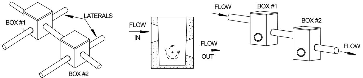
Figure 15: Pressure Distribution Lateral Layout
