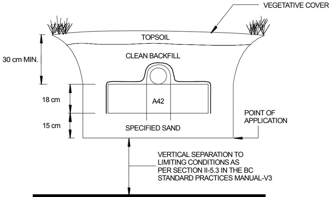
Figure 7: A42 Trench Cross Section
